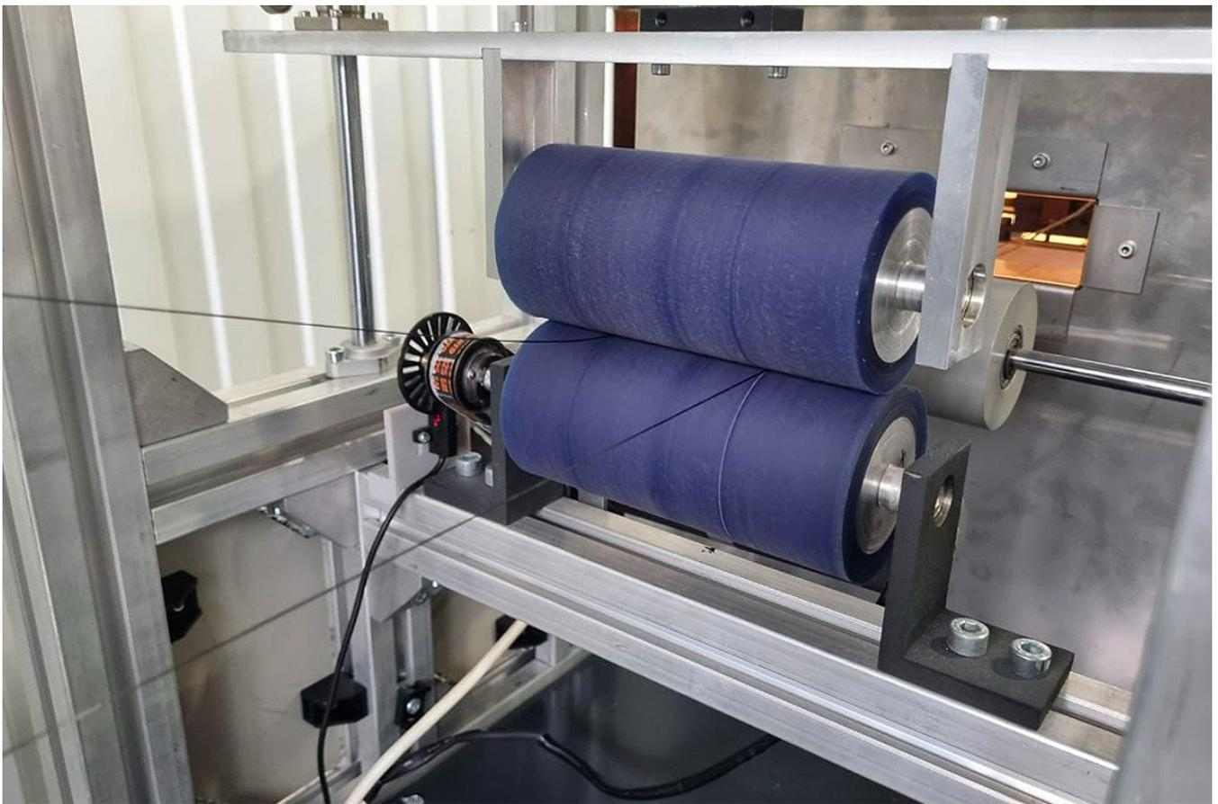
Composite materials (including filaments) from continuous carbon fiber are currently strategic and are practically not exported. Employees of SPbPU Digital Engineering have developed not only the technology for manufacturing filaments from continuous carbon fiber based on thermoplastics, but also manufactured a laboratory unit for its production with a capacity of 500 meters of filament per hour.
