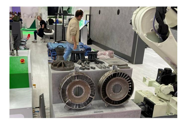
A unique exhibit was the mobile laser surfacing complex «Nomad». The robot is designed for laser cladding of products on the customer's territory.
