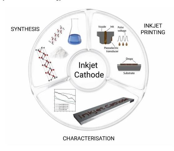
Using the synthesized active cathode material, the scientists prepared a stable colloidal solution and optimized its rheological parameters for inkjet printing. They selected the conditions for printing electrodes, conducted a study of the
