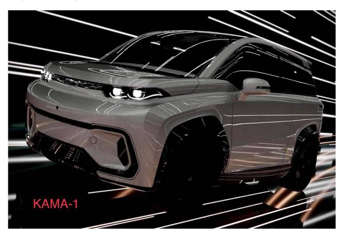
"Kama-1" is a compact urban smart crossover of economy class, capable of driving more than 250 km without recharging, speeding up to 150 km / h and withstanding frost up to  $-50^{\circ}$ C. The car is designed for four passengers, and its price will be about one million rubles with the planned volume of sales of about 20 thousand cars per year.
