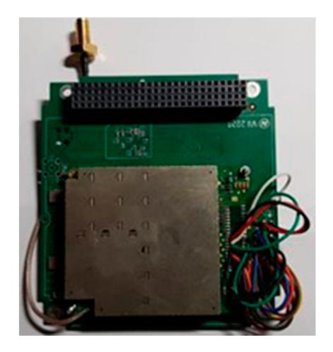
The Institute of Electronics and Telecommunications of SPbPU has developed an AIS receiver (dimensions  $95\times95\times15$  mm). The spacecraft is planned to be launched later this year from the Vostochny Cosmodrome. It should be reminded that SPbPU has already participated in the launch of three microsatellites that successfully completed their missions.
