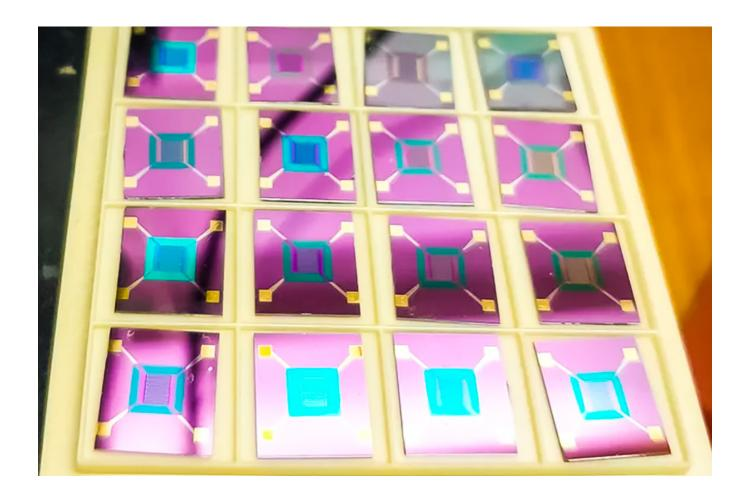
According to experts, this approach increases the sensitivity of the sensor and reduces power consumption, and the used nickel oxide modified with metal nanoparticles, significantly extends the life of the sensor.
